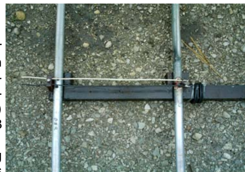
Close-up view of the stub-style feed system
