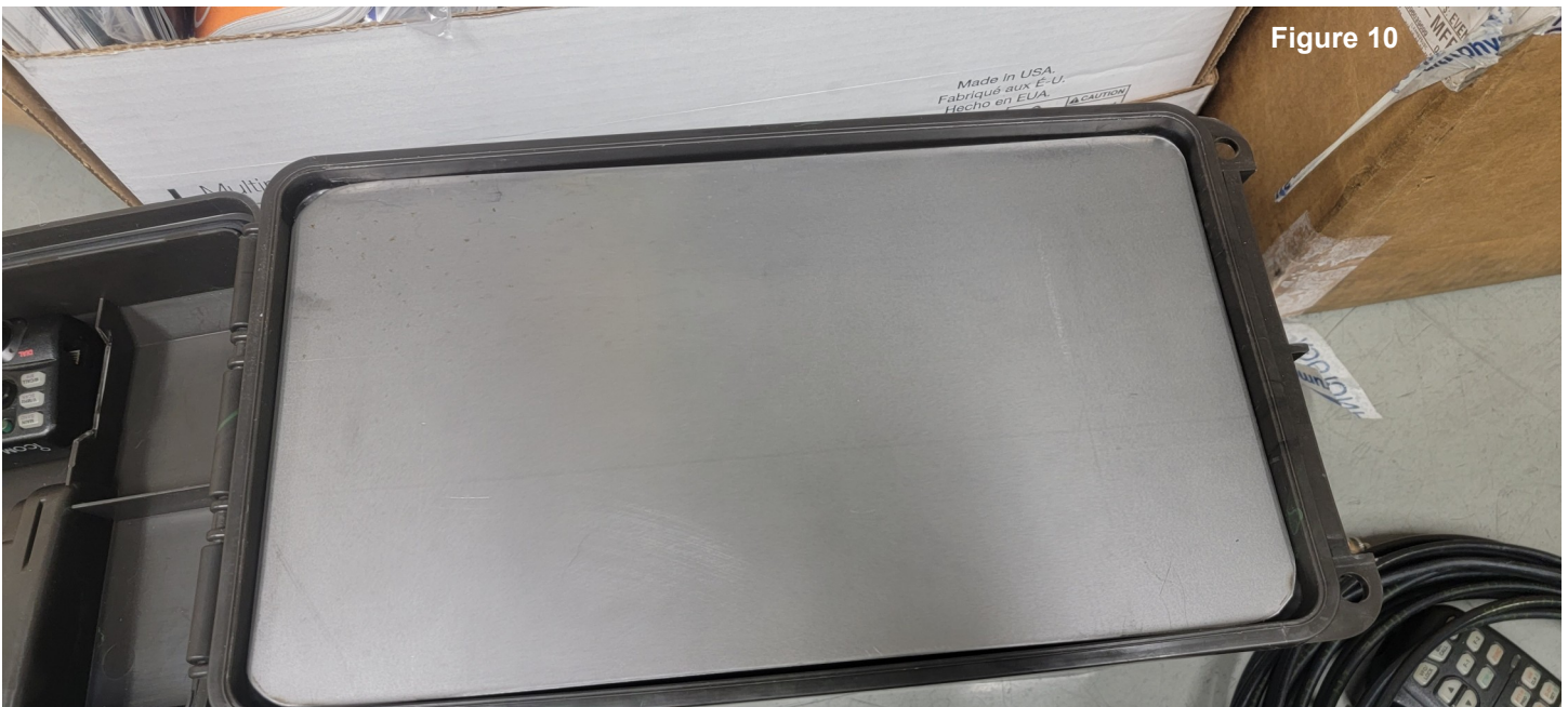
Figure 10: Flat plate fitted on carrying case, before mounting radio, feet and additional finishing
