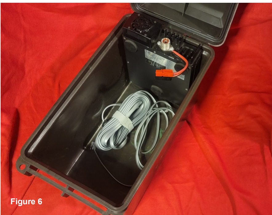
Figure 6: View of radio inside box with remote head cable
