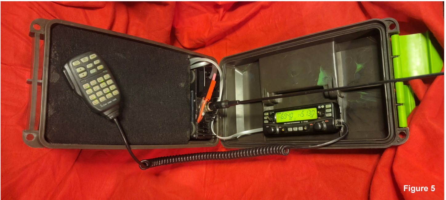
Figure 5: Radio running on battery power with HT whip antenna
