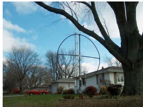
Loop antenna in place. Note that the antenna is mounted in a rotor at the bottom and is not hanging from the tree bough
