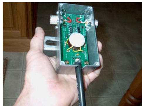
Inside view of the varactor tuning box showing neat layout and straight-forward construction
